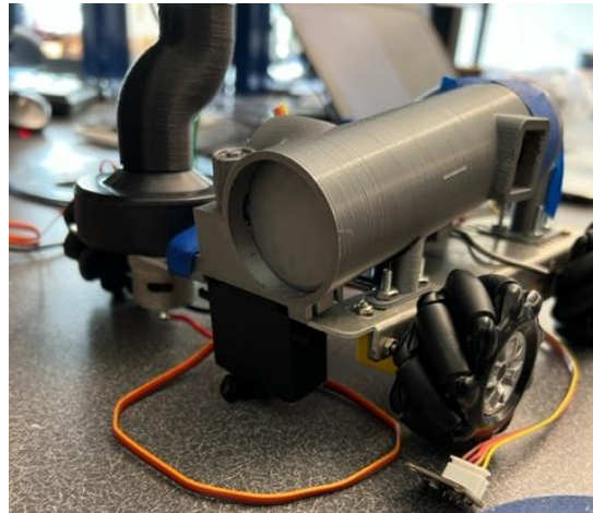
Figure 4. The flapper arm blocking the exit of the processing tube. Balls of the correct color exit on the vacuum side, where a vertical tube would lead to the storage dome.
